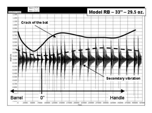
**Figure 2.** Vibration test results for 29.5 oz. RockBat (Lightweight bat). Vibration measured 6-inches from the end of the knob, and impact made at 1-inch increments along the barrel
