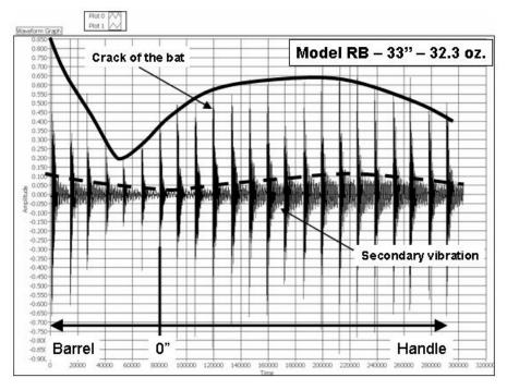
**Figure 1.** Vibration test results for 32.3 oz. RockBat (Heavy bat). Vibration measured 6-inches from the end of the knob, and impact made at 1-inch increments along the barrel
