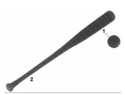
vibration in the batters' grip. This region is commonly referred to as the "sweet spot". There are many definitions of "sweet spot", and what is described here is the vibration form that results when a node of vibration coincides with the batters' grip (2). Because solid-wood bats vary due to the density and stiffness of the wood, the location of this "sweet spot" varies from bat to bat. In other words, no two solid-wood bats are alike.
